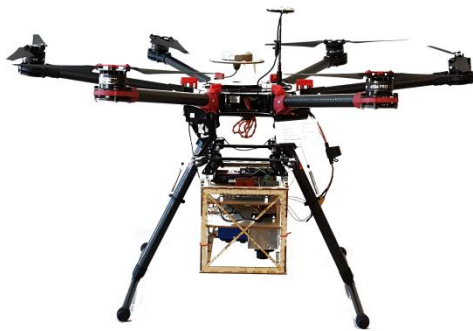
Fig. 1 (a) Hexacopter DJI Spreading Wings S900. The wooden box hosts the UAV payload. (b) The hexacopter during a flight above a lagoon.
