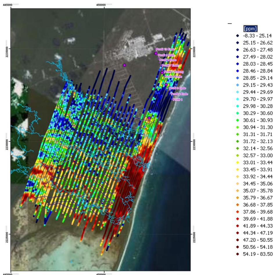
Fig.1: Results of the 7200 Hz inphase component after application of an empirical altitude correction to 70 m of altitude and micro levelling (light blue: known caves; dark blue lines: derived unknown cave branches; purple points: geoelectric profiles 2009)
