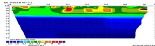
Fig.5: Results of geoelectrical inversion, location of profile near coastline
