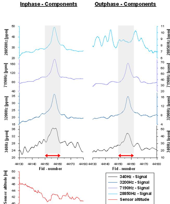
Fig. 3: Results of airborne measurements over a water filled sinkhole (cenote) structure, showing inphase and out-of-phase components and the sensor altitude (red curve) along the flight profile, shaded area indicates position of the cenote
