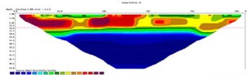
Fig.5: Results of geoelectrical inversion, location of profile: 2 km distance from coastline
