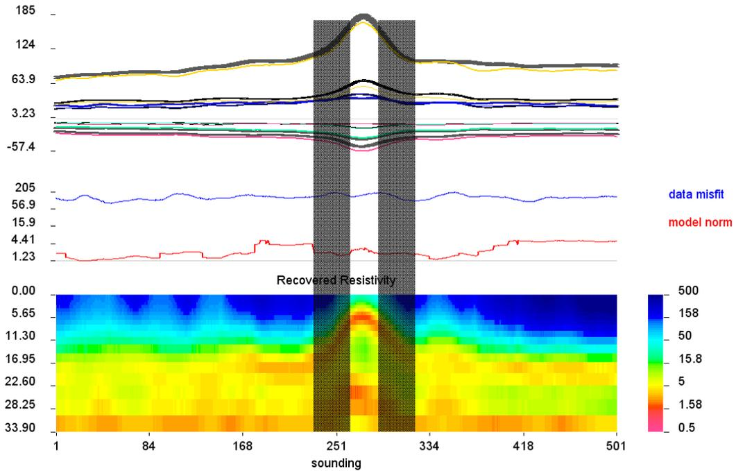
Fig.4: EM Inversion results crossing a known sinkhole structure
