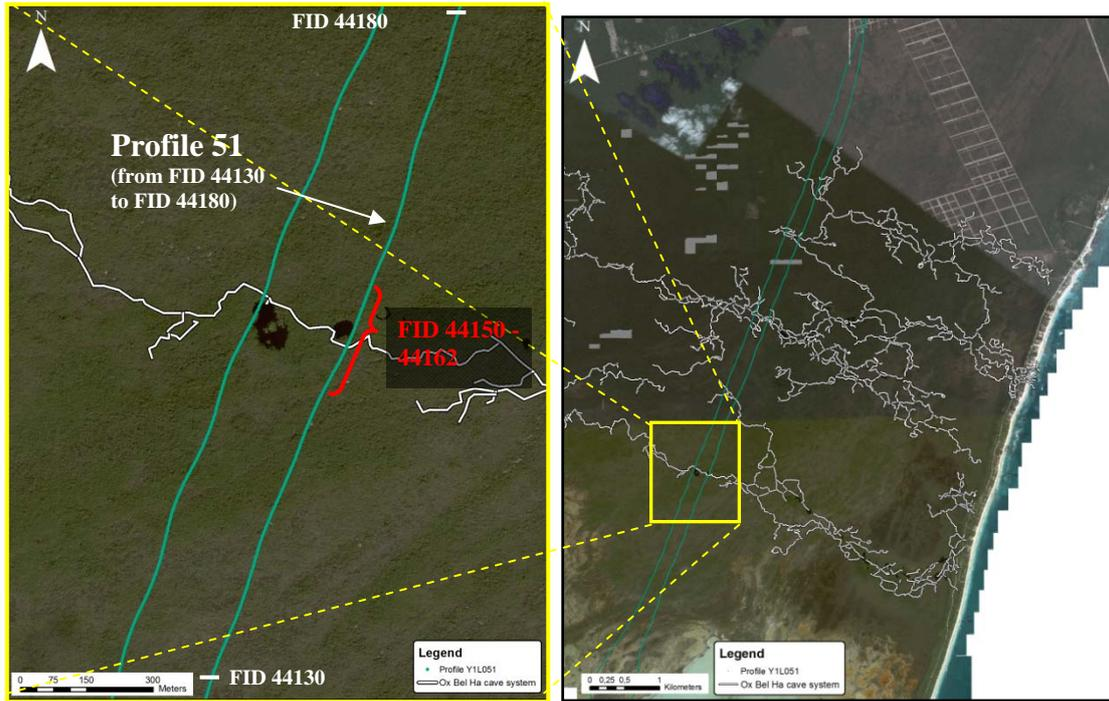
Fig.2: Section of Profile 51 (FID 44130 – 44180) with cave system (white lines) and an overview map of the investigation area
